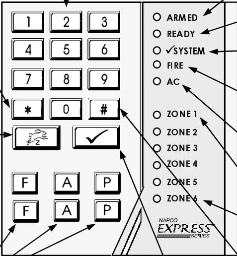
**Armed Light** will light when system is Armed, and will flash when system is in Alarm
