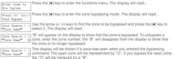
To exit the bypassing mode and return to the Ready state, press the [#] key.
